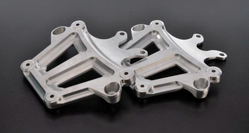
THE CNG SOLUTION CAN DELIVER A WIDE SPECTRUM OF OPTIONS TO SATISFY CRITICAL TEST EVALUATION, AND CAN DELIVER PARTS FAR QUICKER THAN PROTOTYPE METAL CASTINGS. THIS CAN BE ADVANTAGEOUS, AT THE EARLY STAGES OF DEVELOPMENT, IF THE CHOSEN ROUTE TO PRODUCTION IS PRESSURE DIE CASTING, SAND CASTING OR INVESTMENT CASTING FOR INSTANCE. BY OBTAINING AND EVALUATING PROTOTYPE METAL PARTS VERY QUICKLY PRIOR TO COMMITTING TO PRODUCTION TOOLING, RISK LEVELS CAN BE SERIOUSLY REDUCED.
